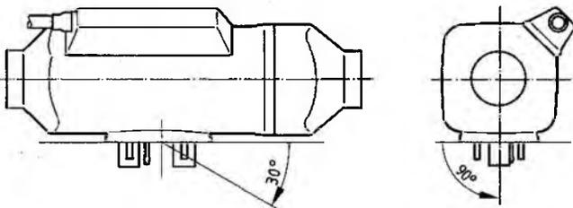
The heater should be installed in the standard position as shown. See sketch for maximum permissible deviations.
