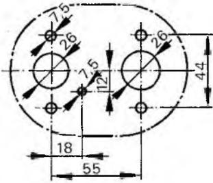
The hole for the cable leading to the metering pump is not included in the template and must be drilled to suit the installation method.
