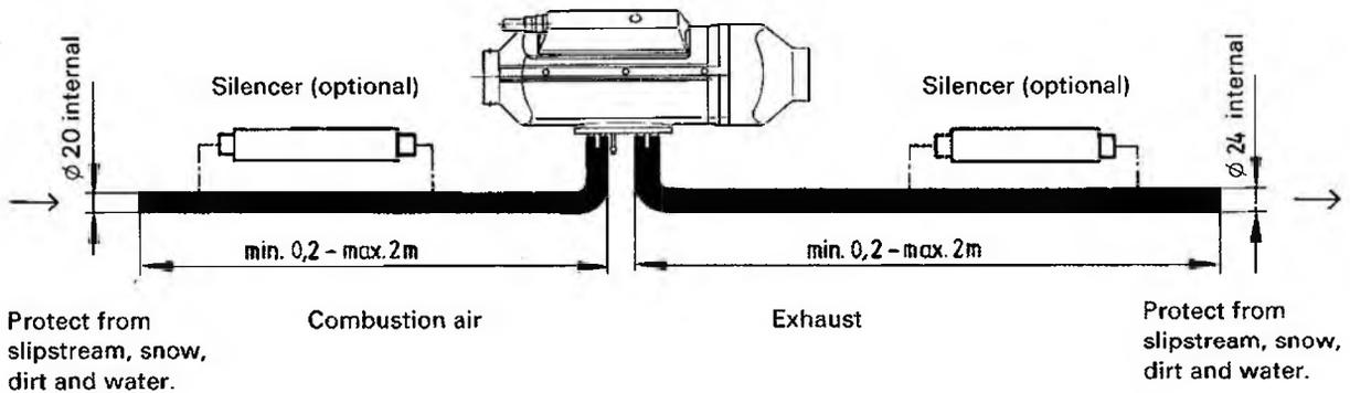
Permissible diversions – exhaust line: max. 180°; combustion air line: max. 180°.
