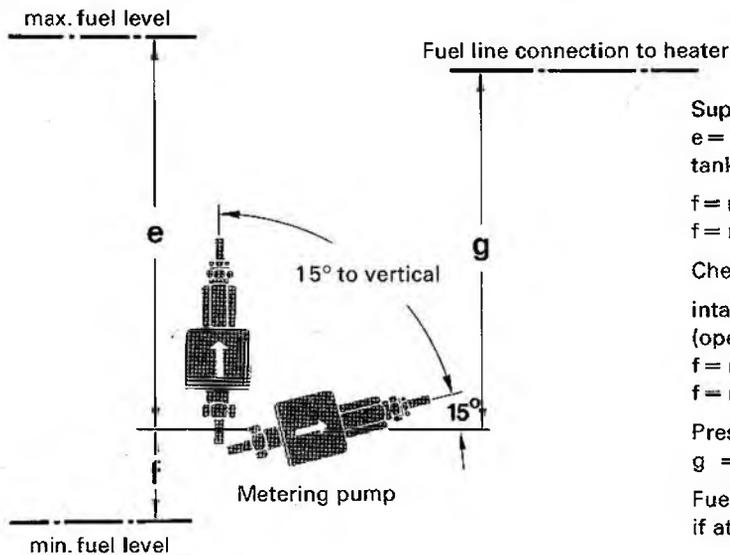
Supply pressure from tank to metering pump:
